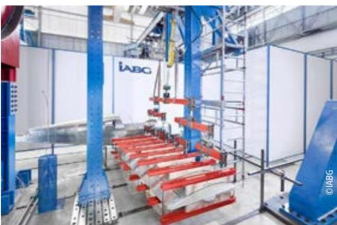
*The wing of the Sonaca 200 on its test bench for limit-load, ultimate and failure load.*
