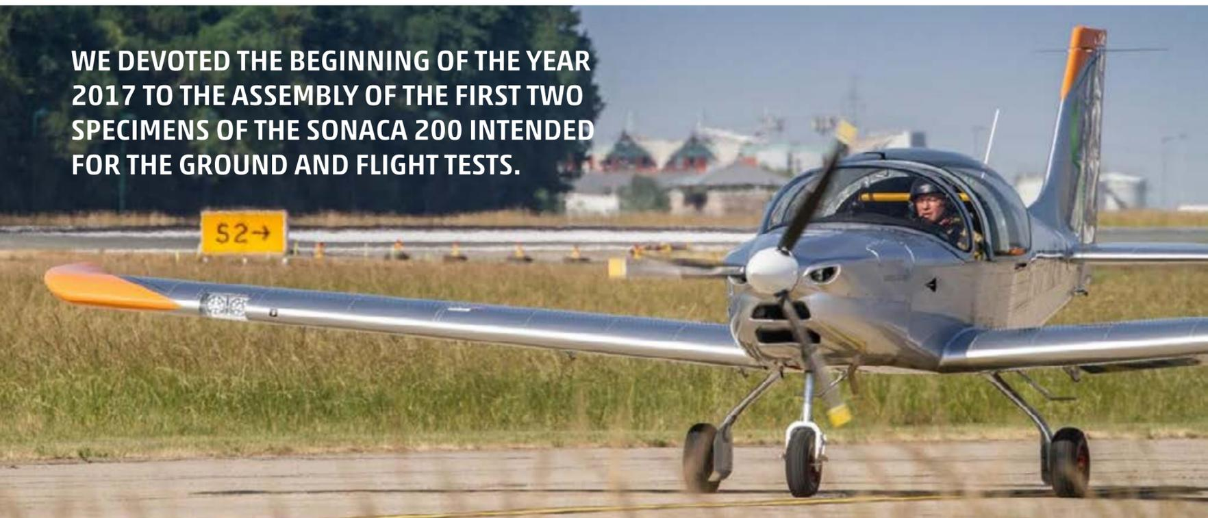
The first aircraft (FTA1, Flight Test Aircraft 1), assembled at Sonaca's site in Belgium, was entirely dedicated to ground tests. We tested the resistance of the seats, the seat-belts (harness) as well as the engine mount and the nose gear leg by simulating hard landings or through crosswind. By the end of February, the wing resistance tests were carried out by the IABG, an aeronautical test centre based in Germany and specialised in resistance tests.
